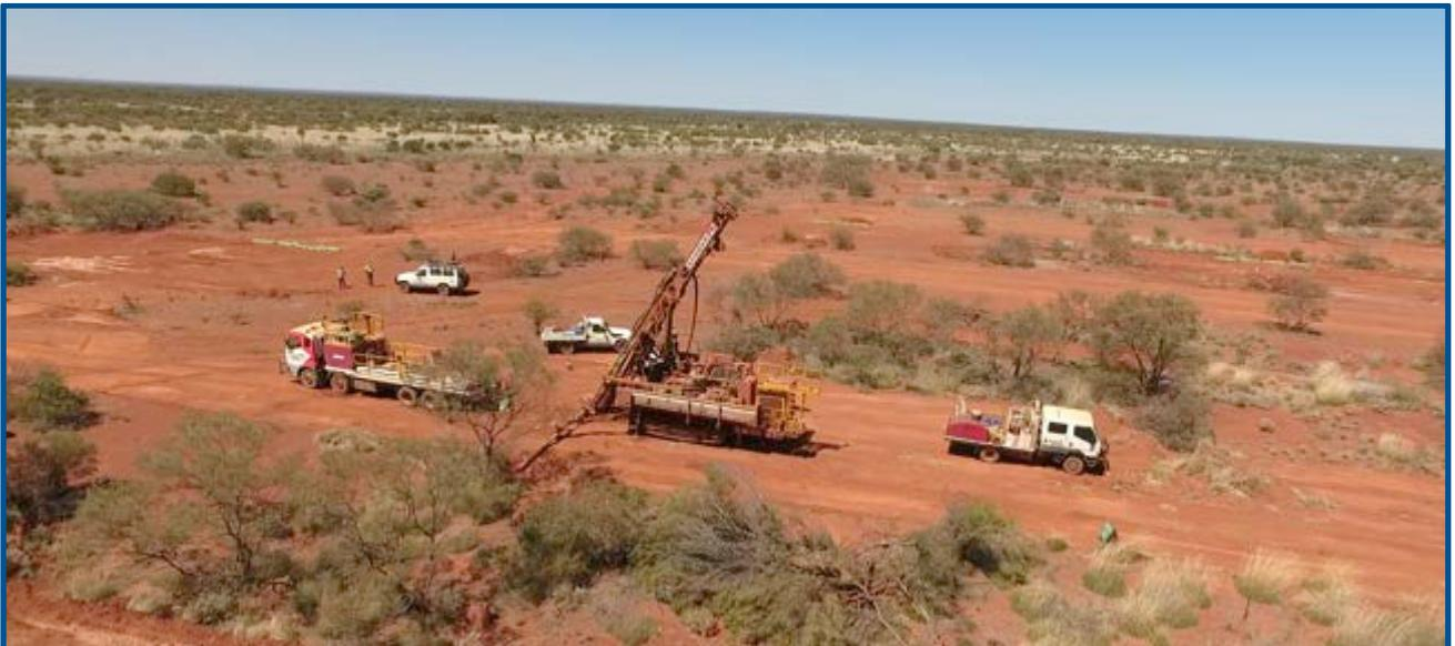
RC drill rig in operation
