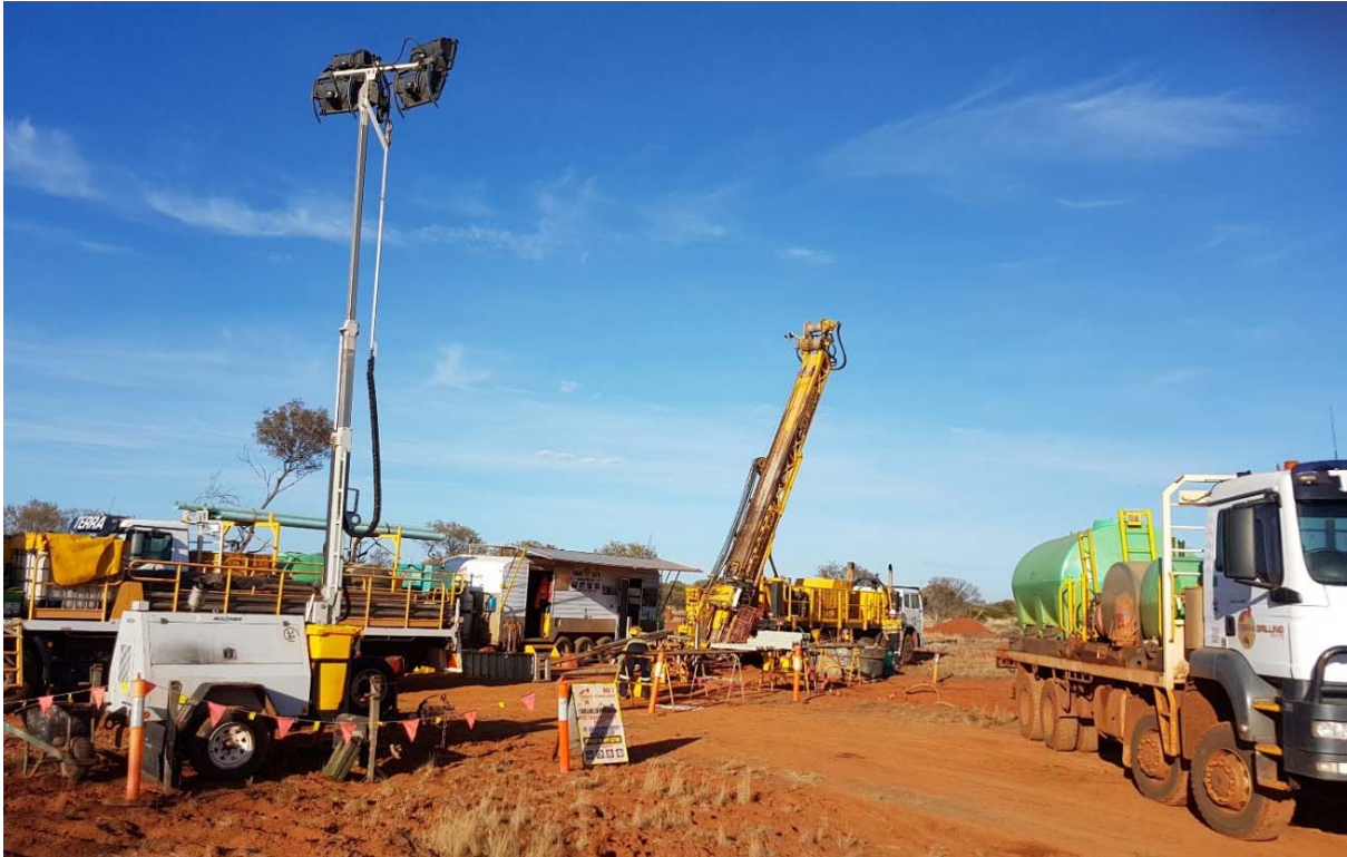
Figure 2. Bibra Deeps EIS deep diamond drilling in progress.
